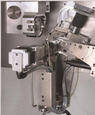
Torque, distance and automatic blade thickness control by microstep clamping
