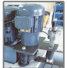
Finish Grinding Unit
