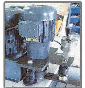
Finish Grinding Unit
