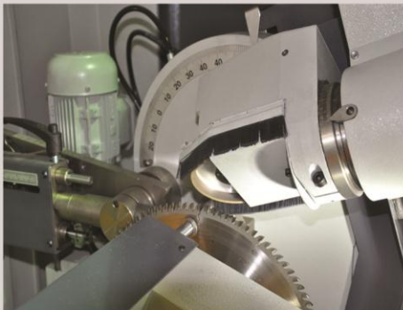
Operator-friendly ABM construction for ease of use. linear bearing system for higher grinding results.
