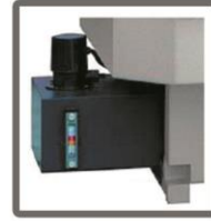
Capacity 100lt coolant container with level indicator
