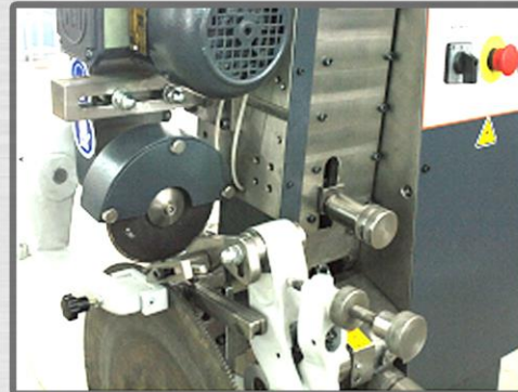
Manual Right / Left Chamfering of HSS Circular Saw Blades
