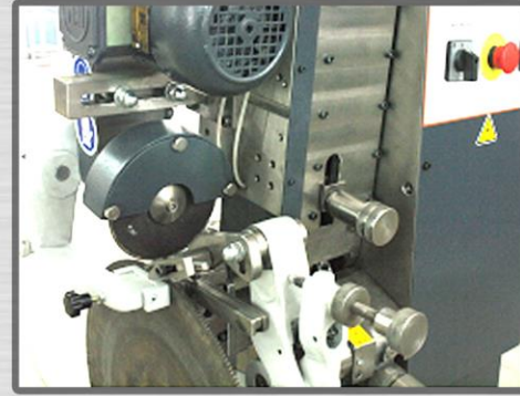
Manual Right / Left Chamfering of HSS Circular Saw Blades
