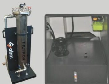
Central automatic lubrication system, optional coolant micro filtration system and optional air filtration system
