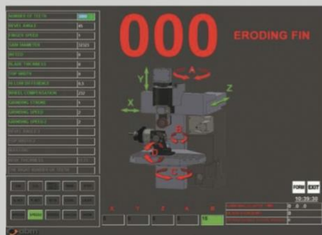
Operator friendly ABM-interface for ease of use. Positioning display of all 6 axes.
