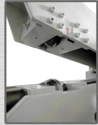
Tensioning rolls providing straightness of camber
