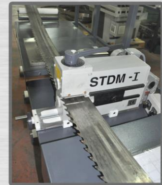
Precise tensioning to prevent possible deflections during operations
